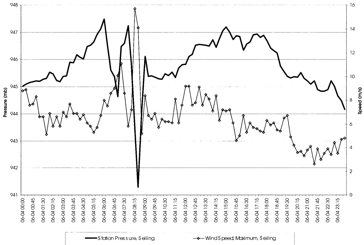
FIG. 8. Pressure spike and corresponding wind gust at the Seiling Mesonet site on 4 Jun 1998.
